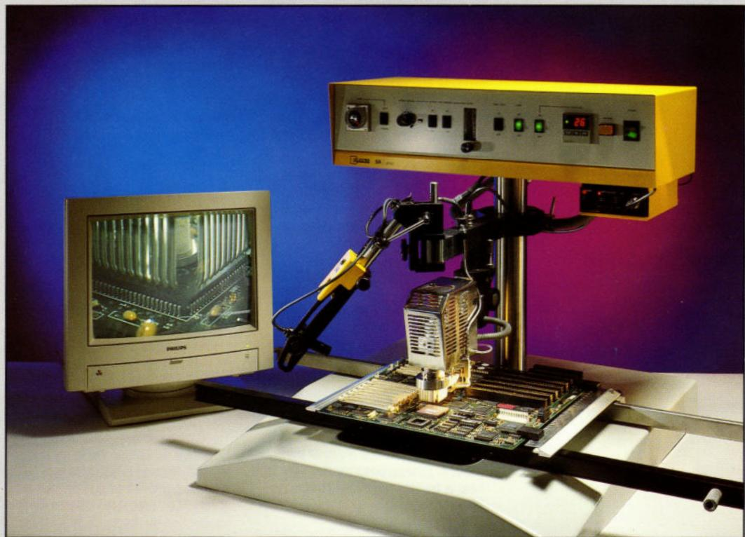
The SR7-100 is a precision hot gas or air PCB component rework system designed to meet the needs of the surface mount and through-hole production environment. A range of products within the SR7 Series is available which can be built up to form a complete rework station.
